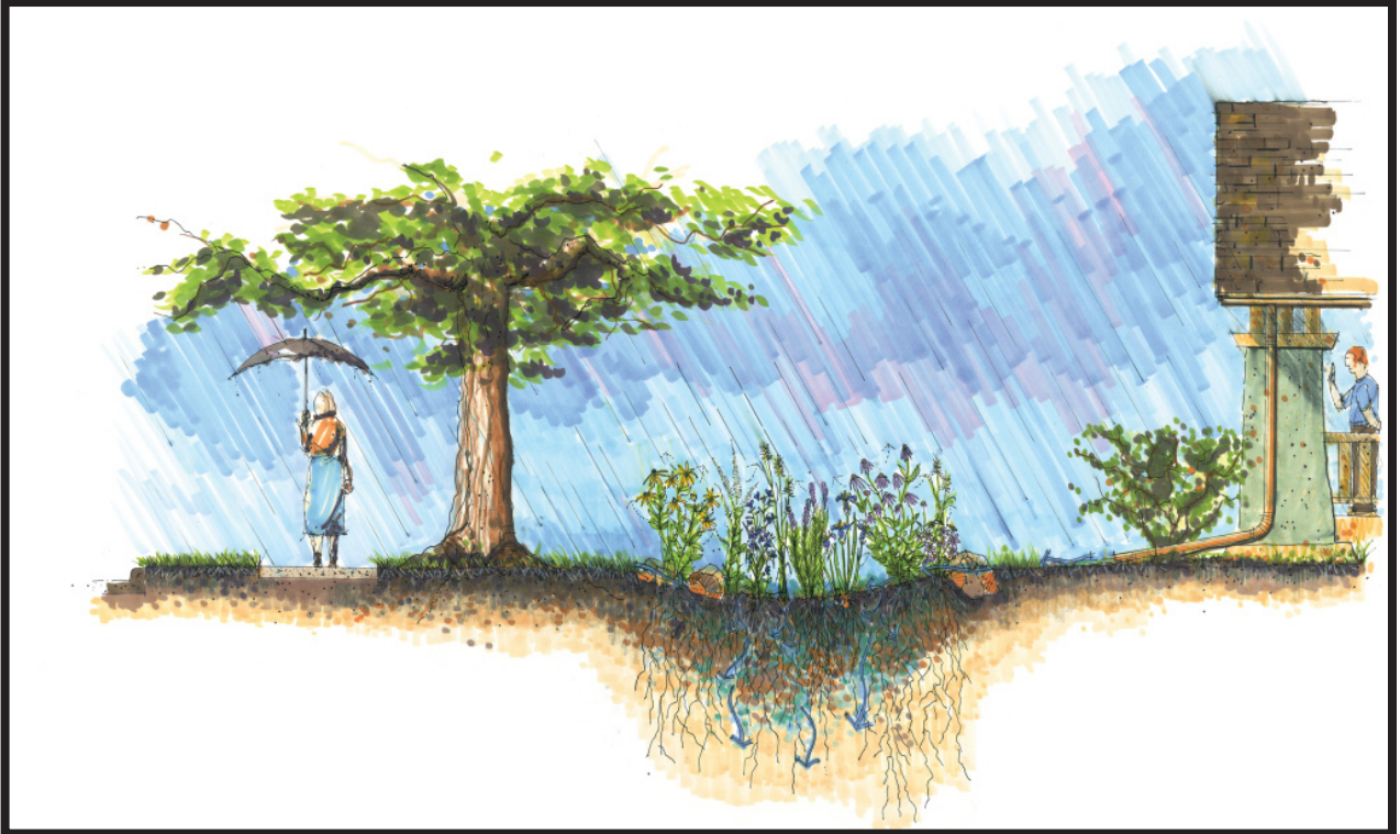
Figure 6.107 Downspout Disconnection to a Rain Garden. Source: Courtesy of USDA-NRCS, Iowa
